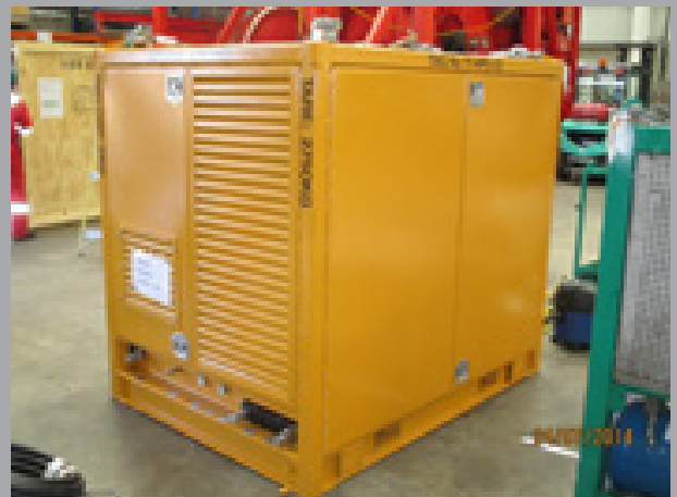
ATEX zone 1 hydraulic power unit (HPU), winch and load monitoring package for production riser pull-in & disconnect
