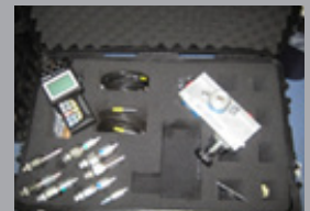
Hydraulic & electrical data loggers, flow meters (0-400 & 0-800 l/min), pressure gauge kits
