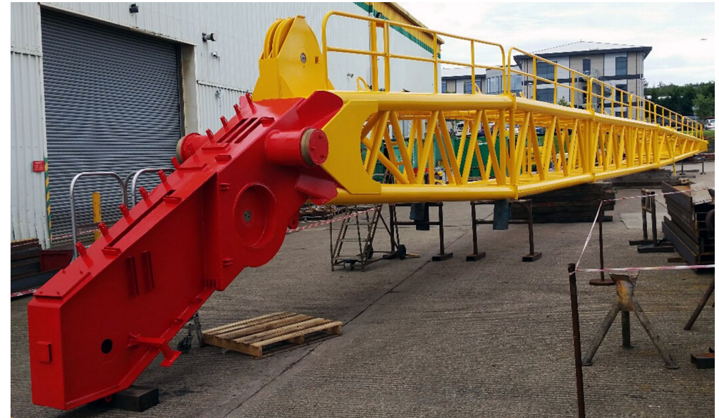
The refurbished and rebuilt boom
